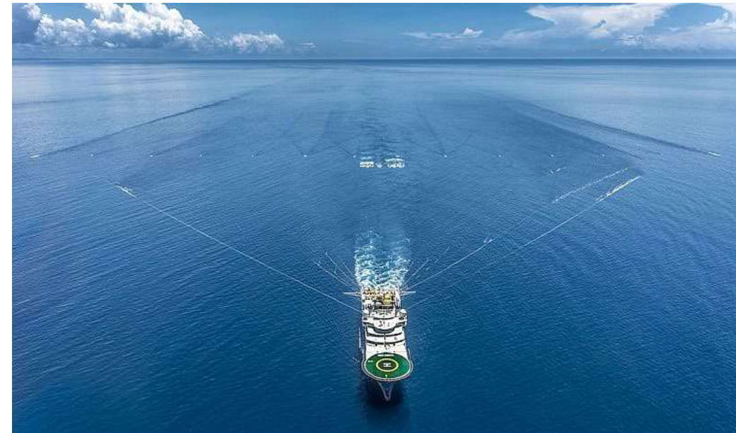
Typical 3D acquisition boat configuration
