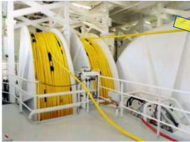
Sound Wave Receivers ("hydrophone streamers")
